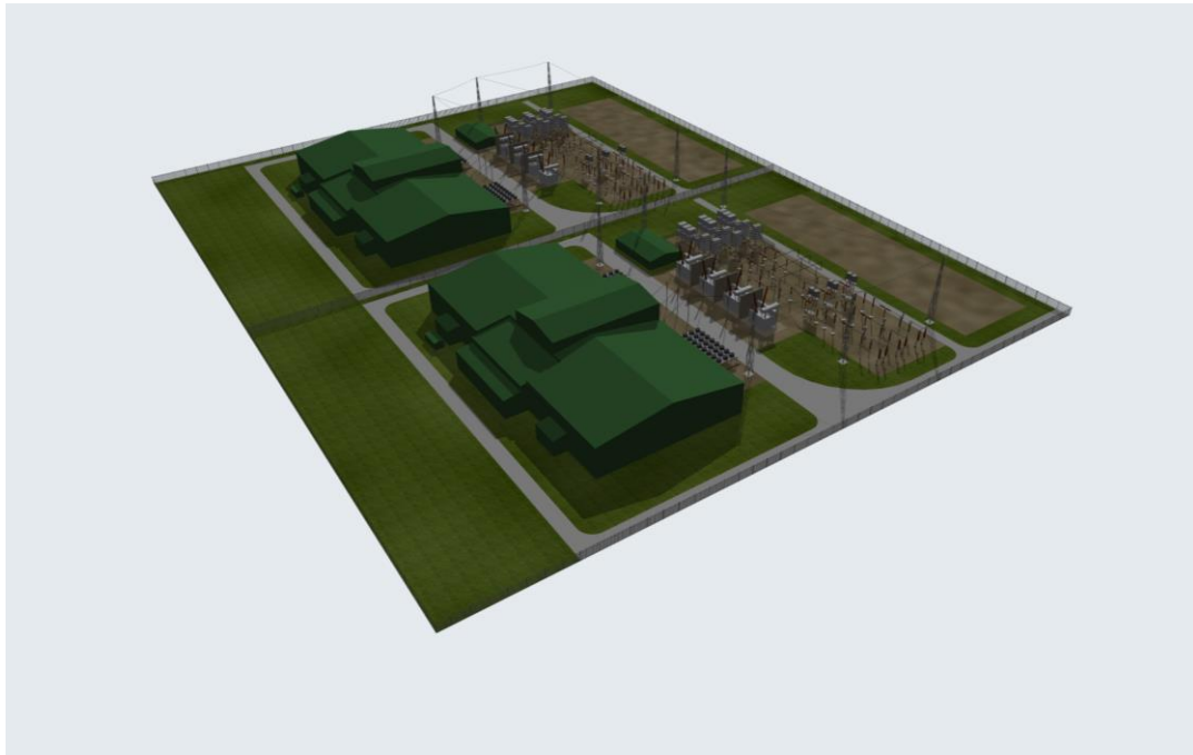
Plate 3 Indicative onshore project substation layout – HVDC
